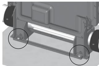
Slide back side of the unit's feet into the guide plate. It should easily slide into place.
