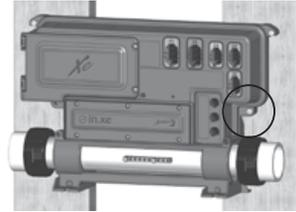
Firmly attach lower mounting holes on each side of the pack with the (2) remaining screws and (2) washers.
