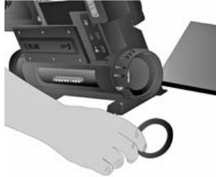
Place a rubber 2" O'ring gasket at the end of each heater nut, to prevent water leakage between the heater nuts and the 2" PVC heater tailpieces.
