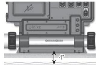
**Note:** The spa pack must be installed at least 4 inches above potential flood level. If floor is on ground level, pack should be raised at least 4 inches.
