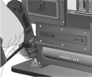
Remove the 2 screws that hold the front of the unit's feet attached to the spa floor.
