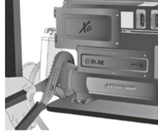
Using an Open-Ended Adjustable Wrench loosen both 2" plastic nuts at each end of the in.xe heater, as illustrated.
