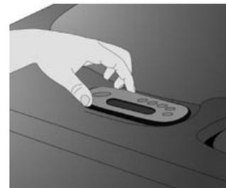
Peel off the double-sided tape protective layer from the back of the keypad.
