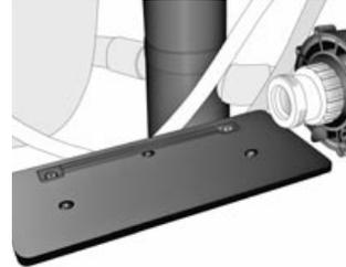
When installing the new in.xe spa pack, slide back side of the unit's feet into the guide plate.
