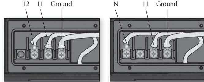
**Connections for 230/240 VAC heater (4KW or 2 KW)**
