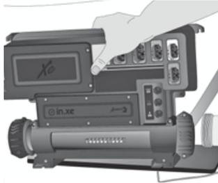
Release the 2" heater nuts from both ends of the spa piping. Release the in.xe Spa Pack by sliding the unit away from the guide plate that holds the backside of the unit's feet in place.
